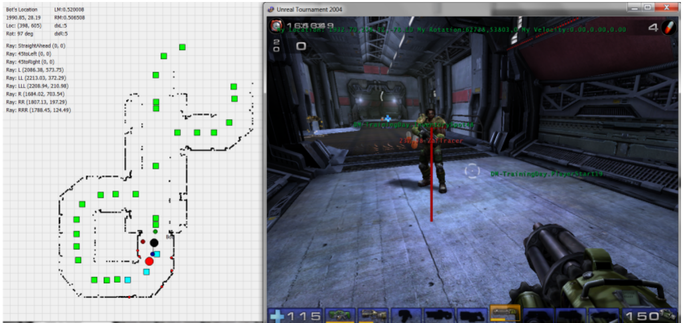
Fig. 2. Game environment. Left: map showing the data available to the bot (black) including other players (red), navigation points both in view (cyan) and out of view (green), as well as wall locations gathered from ray tracing. Right: the in-game view showing an external view of the avatar.
