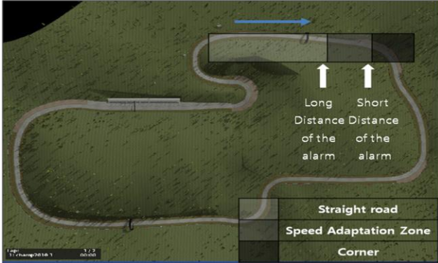
Figure 6. Speed adaptation zone before the corner (the area between two vertical arrows)
