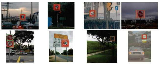
Figure 3. The experimental results of the proposed method which covers weather, illumination effects, and occlusion (The red rectangle expresses the candidate, the green rectangle represents the final decision)
