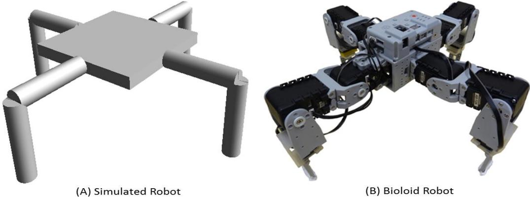
Figure 2. Physical Design of a Quadruped Robot
