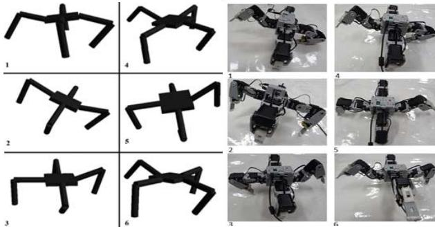
Figure 4. Simulated and Bioloid Quadruped Robot Movements
