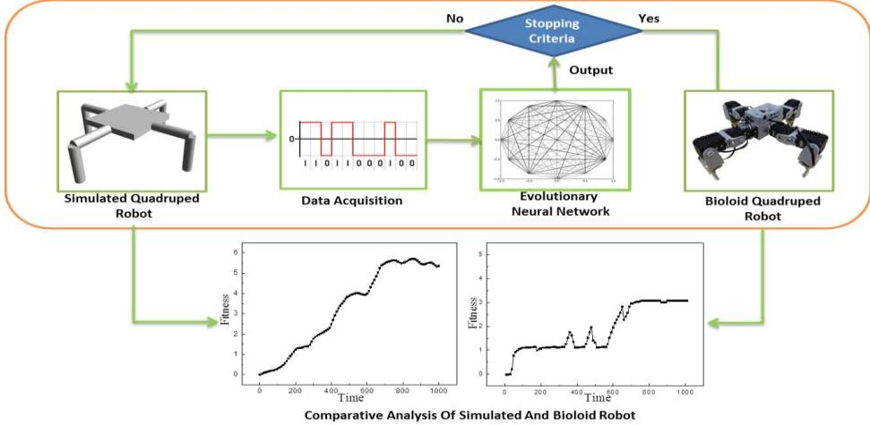
Figure 1. An Overview of Analysis and Comparison of Simulated and Real Quadruped Robot
