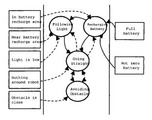
Figure 5: Behavior network of Khepera mobile robot in this experiment.
