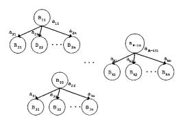
Figure 2: Behavior search tree selects maximum n behaviors and processes from root to the k-th level. We can acquire maximum  $n^k$  behavior sequences at the level.
